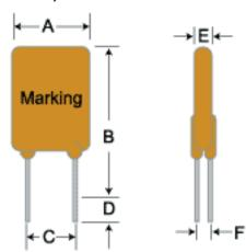
Lead Size RG300-16~RG1100~16 Ø 0.81 mm Diameter 20AWG Lead Size RG1200-16~RG1400-16 Ø 1.0 mm Diameter 18AWG
